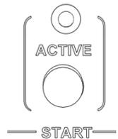
3) The stimulation ACTIVE light will first flash for a period of approximately 30 seconds while the current is ramping up. The TRUE CURRENT™ display will show the current ramping up to the set INTENSITY value. For waveforms with frequency content (PCS, ODCS), TRUE CURRENT™ indicates the maximum value the waveform is able to reach.
